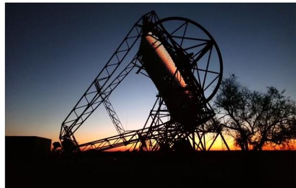
H.E.S.S. is a system of imaging atmospheric Cherenkov telescopes dedicated to observing the most violent and extreme phenomena of the universe in very high energy gamma-rays (in the
